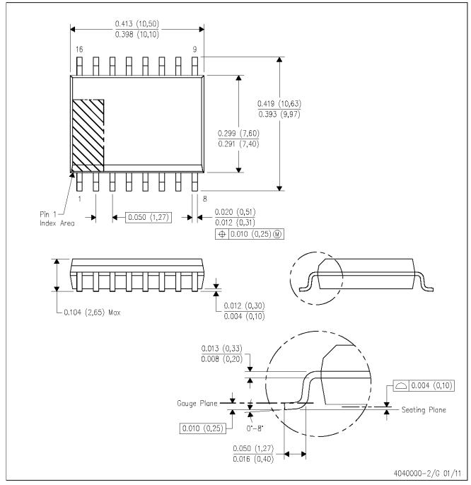
NOTES: A. All linear dimensions are in inches (millimeters). Dimensioning and tolerancing per ASME Y14.5M-1994.
